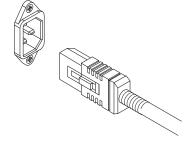
The V-LOCK power cord has a special latching feature to prevent the power cord from being unintentionally removed. The IEC plug and socket are both blue in color so the power cord can be identified as a KW Series loudspeaker cord. If the QSC supplied cord becomes lost or damaged, a standard replacement 18 gauge IEC power cord may be used. However, the latching system functions only with a V-LOCK power cord available from QSC Audio Products, LLC.
