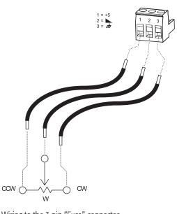
Wiring to the 3 pin "Euro" connector.
