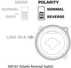
When using only one KW181 and connecting a LEFT and RIGHT stereo signal, start with the polarity switch in the NORMAL position. With the system at a reasonable level, change the POLARITY switch and evaluate which polarity results in the most low-frequency output.
