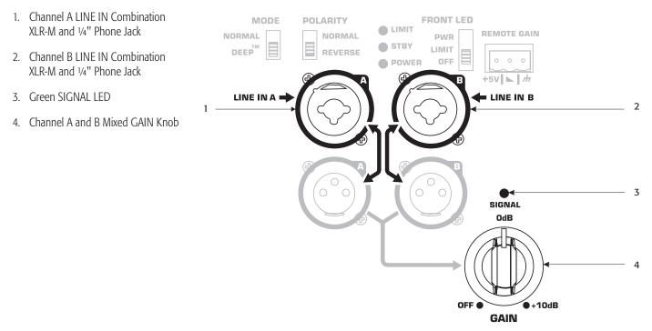
The green SIGNAL LED illuminates when a signal is present at either input, regardless of the amount of gain as set by the GAIN knob. If the LED does not illuminate, the input is not receiving any signal, or the level of the signal is too low. Check all connections and the status of the device delivering the signal.
