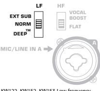
KW122, KW152, KW153 Low-frequency EQ Switch
