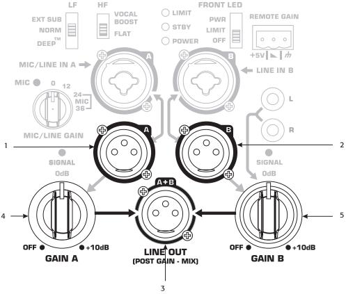
Both Channel A and Channel B have discrete, direct outputs on female XLR connectors. The signal on this output is exactly equivalent to the signal from the corresponding input. The level of the output signal is not affected by the gain setting for that channel. If a unit is OFF, any signal present on MIC/LINE IN A or LINE IN B passes through to the respective discrete outputs. Any audio signal present on the RCA (phono) jacks does not get passed to the discrete outputs.
