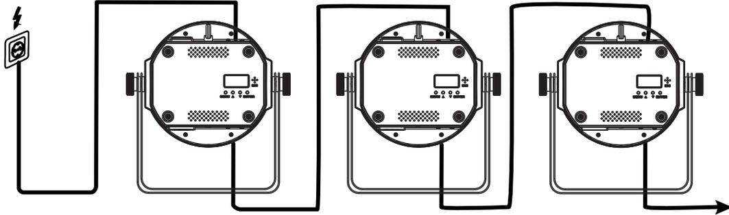
The device uses an auto-range power supply that accepts input voltages between 100 und 240 volts.
