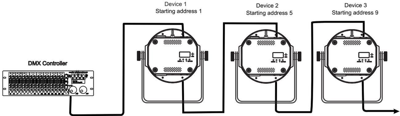
A DMX512 data link is required in order to control the device via DMX. The device provides 3-pin XLR connectors for DMX connection.
