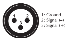
DMX-input XLR mounting-plug:
