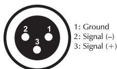
DMX-output XLR mounting-socket:
