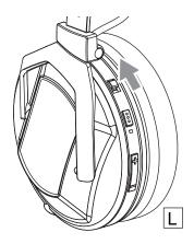
5 With the power turned off, press and hold the multifunction button on the headphones until the connection indicator LED blinks (white).
