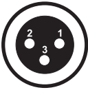
DMX-output XLR mounting-socket:
