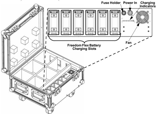
The Freedom Flex Case is an auto-ranging power supply and it can work with an input voltage range of 100 to 240 VAC, 50/60 Hz.
